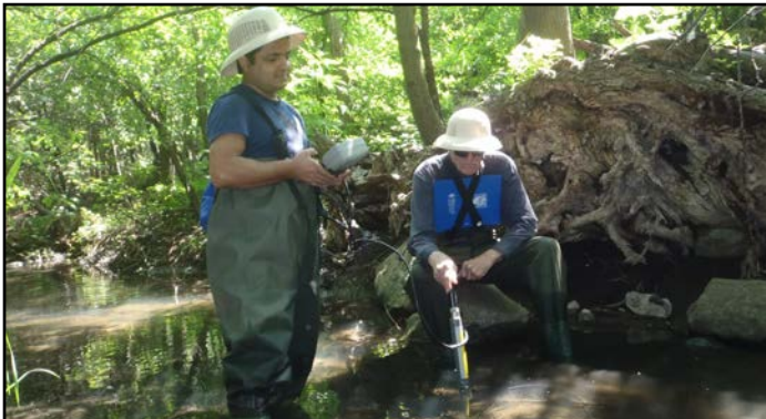
Volunteer collecting water chemistry measurements with a multiparameter YSI probe
